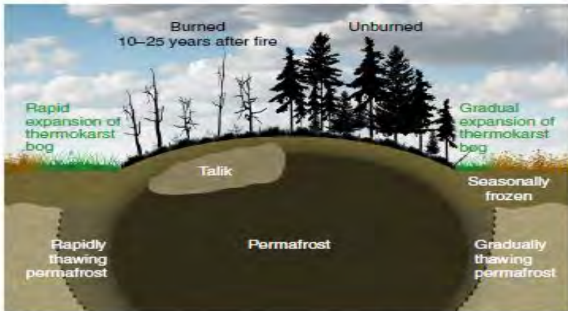
Fig. 2 Simplified illustration of soil thermal states for peat profiles along transects from thermokarst bogs to peat plateaus, within and outside historical burn areas. Taliks are continuously thawed soil layers between the permafrost and the seasonally frozen layers
